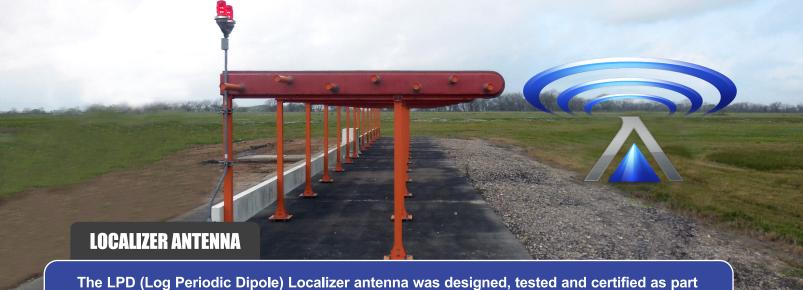
The LPD (Log Periodic Dipole) Localizer antenna was designed, tested and certified as part of the ILS (Instrument Landing System) used to help pilots navigate a successful aircraft landing. Typically deployed in configurations of 14 or 20 units at the end of the runway, the LPD's work with the ILS beacon to provide information to the pilot telling them if they are left or right of the runway.
